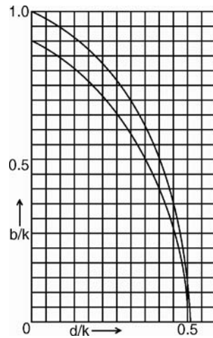
Fig. 5.2. With a certain choice of distance d and slot width 2b of Herzog shunts in relation to plate distance 2k of electric sectors the effective field length coincides with the real one. The curves show b as function of d for thick ( upper curve ) and thin ( lower curve ) Herzog shunts
